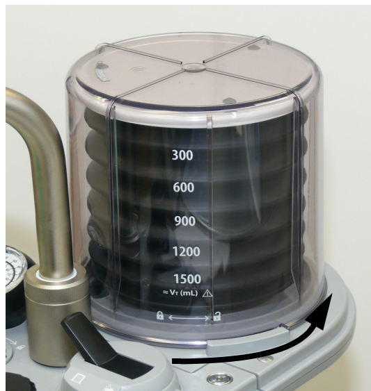
FIGURE 7-5 Removing the Bellows Dome
