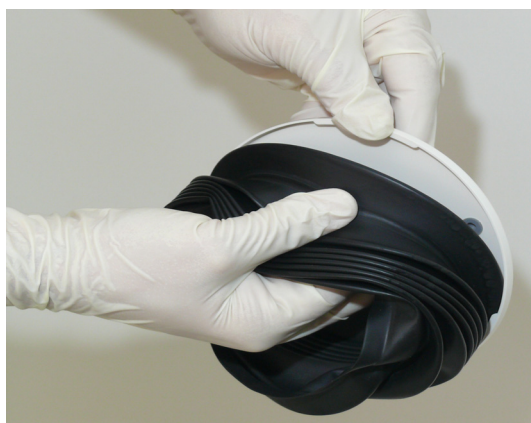
FIGURE 7-7 Detaching the Bellows Top Plate
