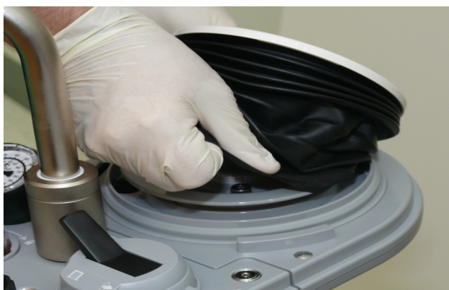
FIGURE 7-6 Detaching the Bellows
