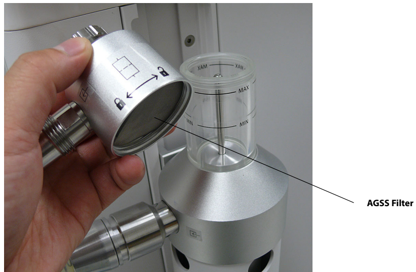
FIGURE 7-24 Removal of AGSS Top / AGSS Filter Inspection
