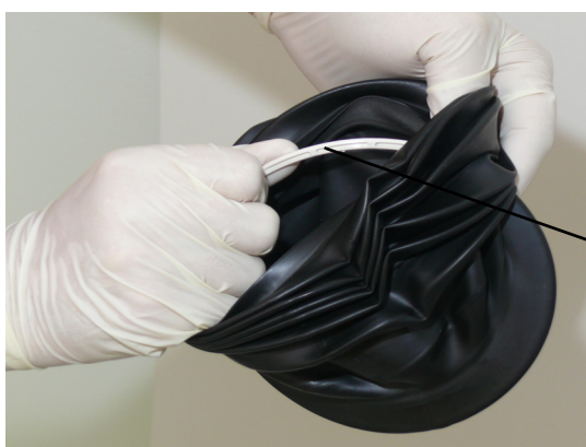
FIGURE 7-8 Removing the Bellows Adapter Ring
